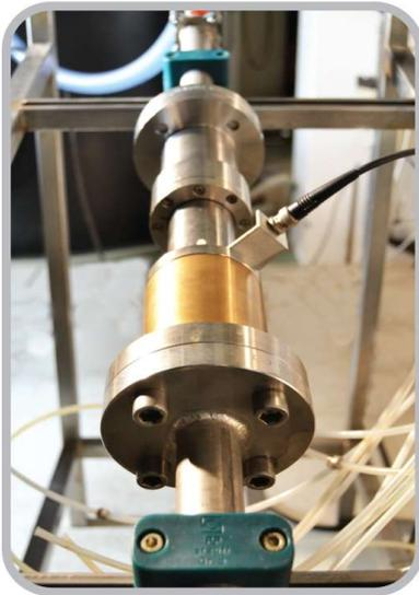
VAG+ consists in a venturi device on which it is possible to relate critical pressure and nuclei sizing. Each activated nucleus causes a cavitation bubble to be formed. After a growth phase, cavitation bubbles implode and create a brief shock wave which is detected by a piezo-electric sensor. Due to an appropriate measurement device, VAG+ allows nucleus counting in a fluid. Then, it is possible to know the dissolved gas concentration, especially during cavitation tests.
