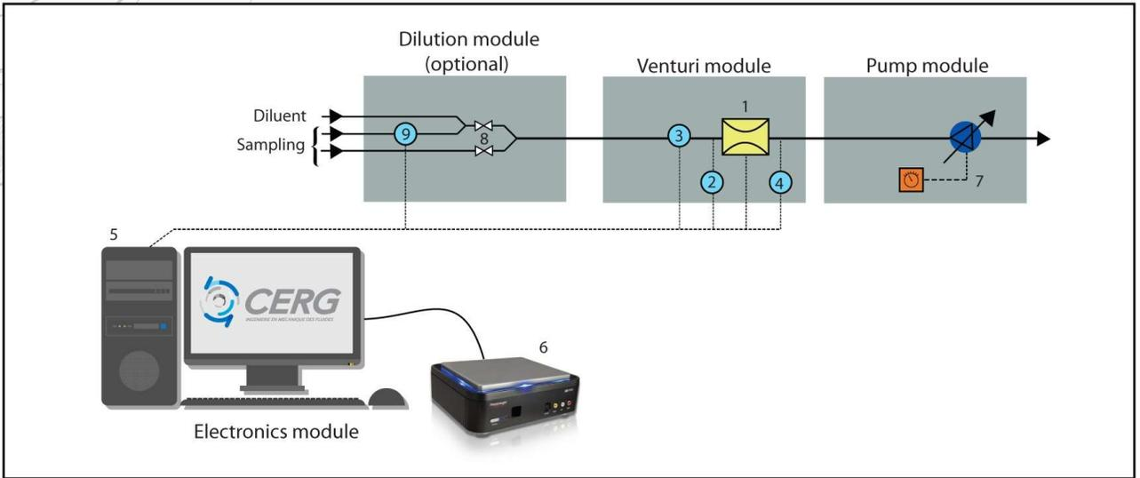
The VAG+ system is composed of 4 modules :
